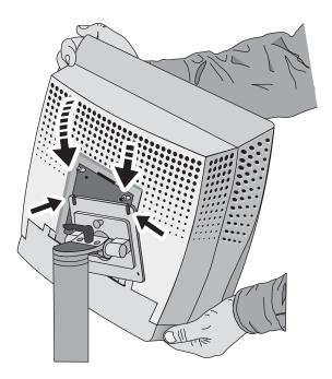
**3** Tighten the top two screws through the fixture's mounting plate.
